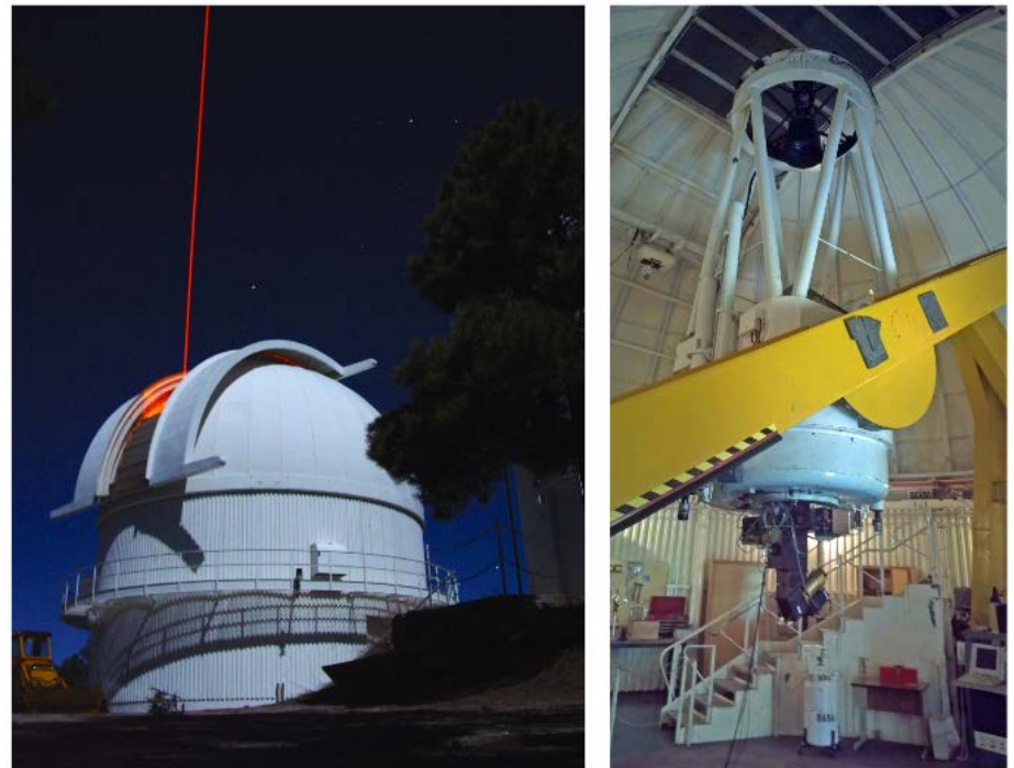
Figure 2. Left, the Kuiper Telescope dome on a moonlit night, with guidestar in operation. Inside the dome, on the right, the Kuiper Telescope used to receive the signal from the sodium layer.
