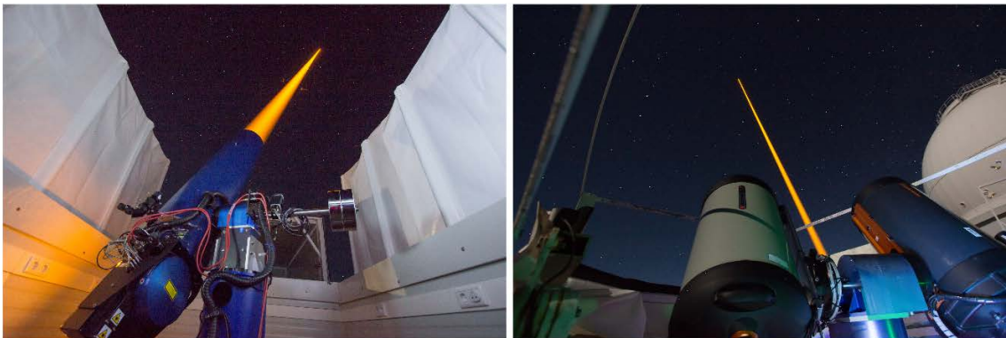
Figure 7: (Left) The 20-Watt laser projector of the European Southern Observatory laser guide star system. (Right) The observing telescope placed next to the laser projector for detection of LGS brightness enhancement.
